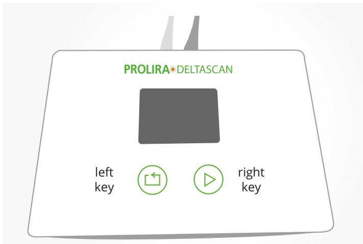
Figure 5: Location of the two keys on the Monitor.
