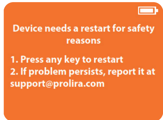
Figure 36: Monitor screen displaying that the device needs a restart after charging.
