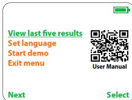
Figure 36: Monitor screen of device menu (available after simultaneously pressing both keys for 3 seconds).
